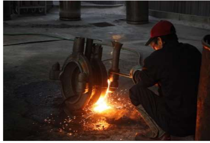
Gas Cutting arc air gouging
