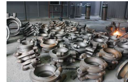
Blast Cleaning (After Blast)
