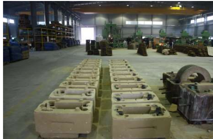
Completed CO 2 Molding
