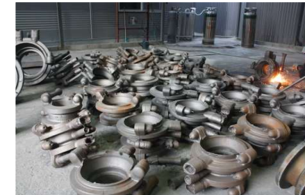
Blast Cleaning (After Blast)
