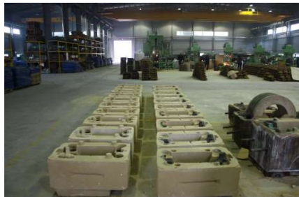
Completed CO 2 Molding
