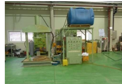
Vertical Hydraulic Press 65 TON
