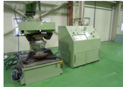
Vertical Hydraulic Press 100 TON
